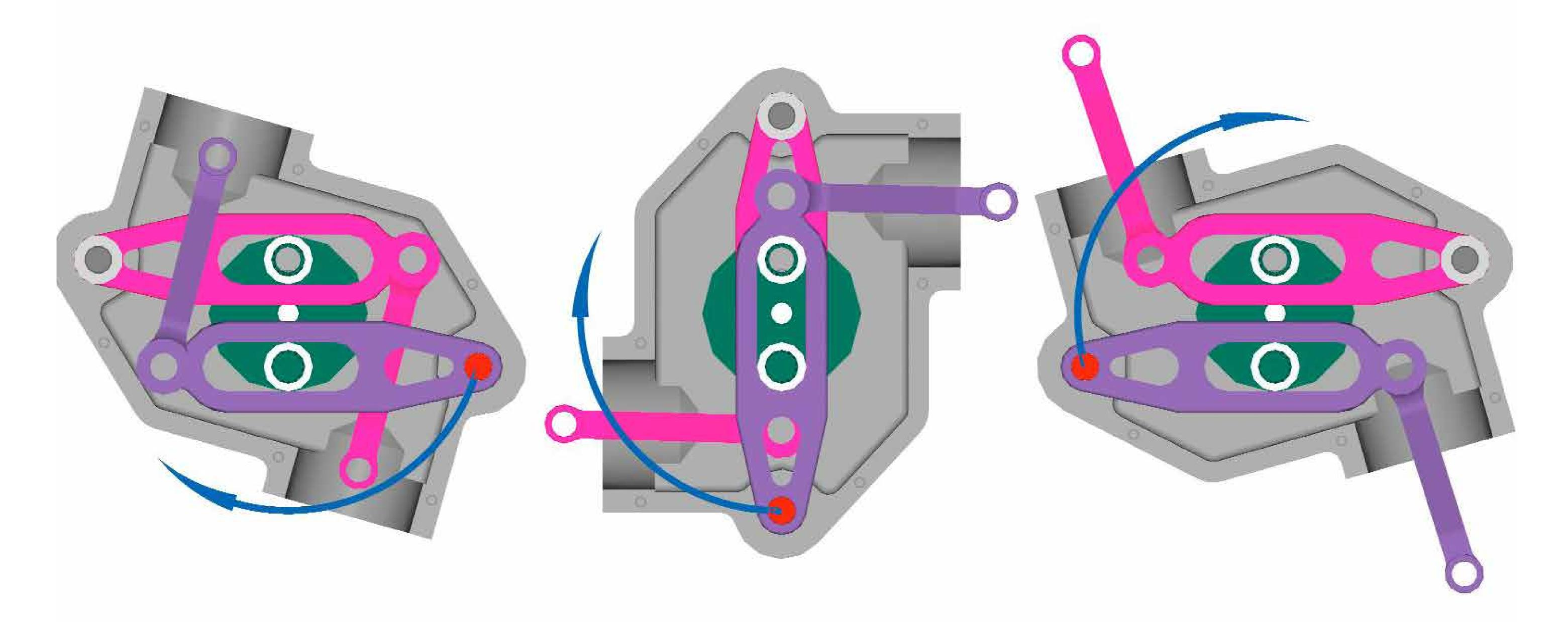
The rotation around the crank's eccentric journal, produce the oscillation of the free arm of the lever and as a result the linear movement of the pistons.
