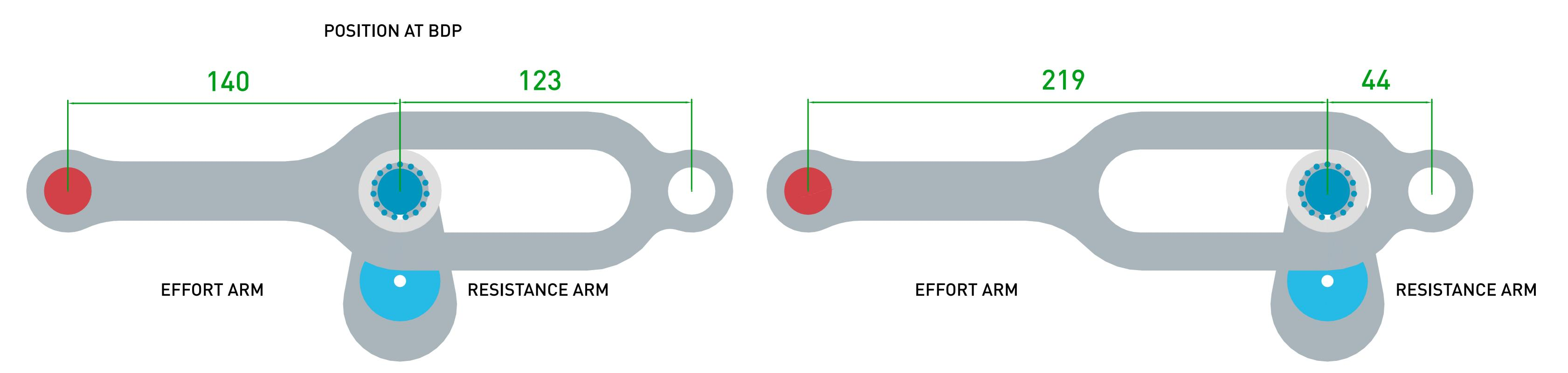
When an external force is applied, by means of a motor or another source, it multiplies the received potency, and consequently reduces the required force to carry out a task.
